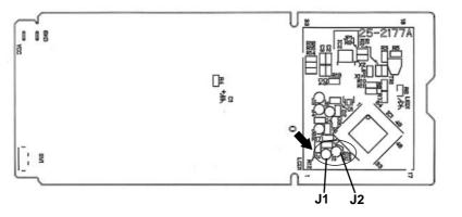
NOTE : For modification, take out the batteries and press the OPERATE/ STOP (ON/ OFF) button 2 or 3 times at first. After modification, put back the batteries then press the RESET button.
